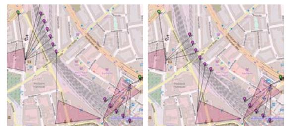
Fig. 2: Handover of a group of users moving along a railway track. The background image shows the central station of Hannover (OpenStreetMap)
