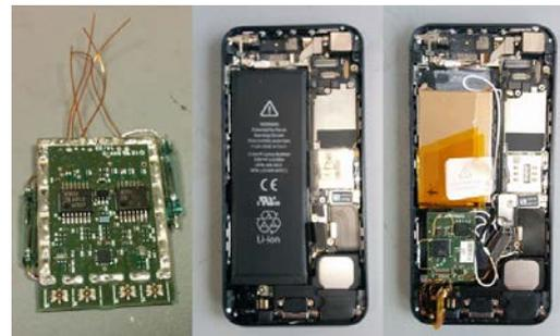
Fig. 1: The TINA (left), the standard iPhone 5 (middle) and the proof of concept phone (right). The measurement concept requires modifications to the phone battery and cabling to make room for the TINA.
